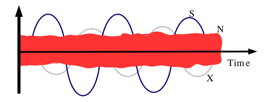
The sum of all fresnelzone-reflected waves adds up to noisefloor N, reducing our Signal-to-Noise Ratio.
