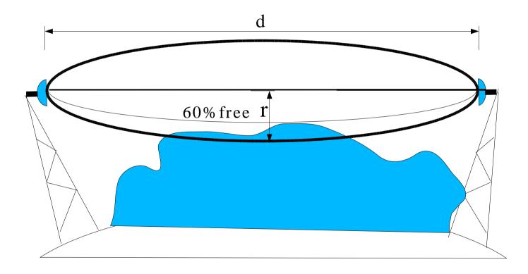
Ideally would be a 80%-free Fresnel Zone, no significant signal loss. Keep at least 60 % of the Zone free – that will sacrifice some signal strength.
