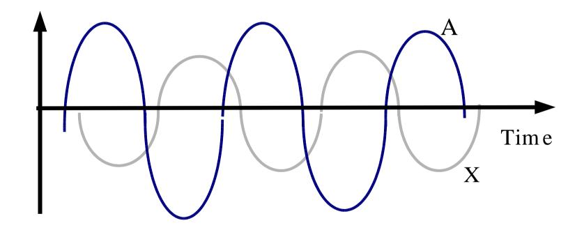
Wave A is the signal we want to receive, following line of sight Wave X is one disturbing wave reflected in the fresnel-zone Wave X is out of phase because it arrived later travelling a longer path.
