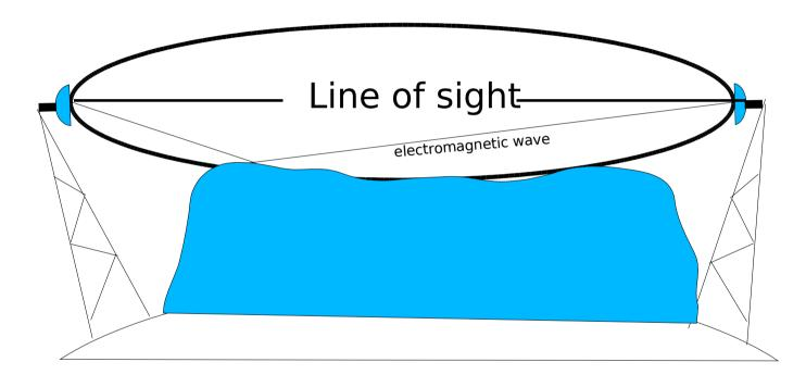
An area between the antennae that looks like a ellipsoid in 3D. If there are objects in this area, electromagnetic waves are reflected and reach the antenna on the receiving side in or out of phase. This will attenuate the signal. (In theory it can also amplify it, though. I promise – it won't...)
